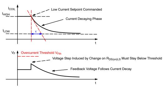
Figure 2. Coil Current Decay when Low Levels are Commanded
