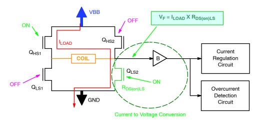
Figure 1. Current Measurement Performed by AMIS-3052x/NCV7052x on One of the Two Stator Windings
